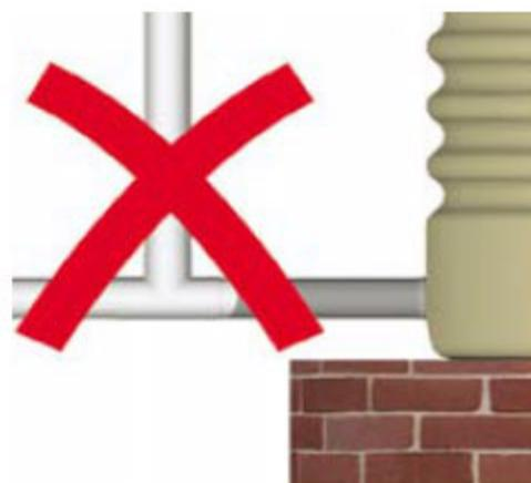
Unsupported pipe work puts excessive strain on fittings and tank wall.
