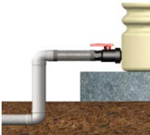
Insert length of flexible pipe to absorb shocks and movement of pipe fittings from tank. Position pipe directly into ground to avoid running over pipe and damaging fitting and/or tank.
