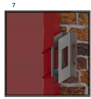
INSTALL NEXT TANK BRACKET DIRECTLY ADJACENT PREVIOUSLY INSTALLED BRACKET DYNABOLT INTO POSITION. IT IS IMPORTANT THAT ANCHOR DOES NOT PROTRUDE MORE THAN 20MM TO PREVENT POSSIBLE DAMAGE TO TANK
