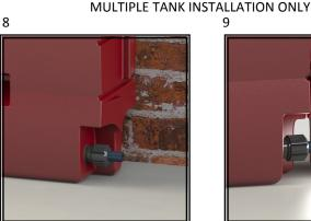
ATTACH BLUELINE COUPLING TO EACH TANK. INSERT BLUELINE TO INSTALLED TANK AND WRENCH TIGHTEN TO SECURE.
