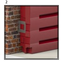
INSTALL BRACKET OVER THE HIGHEST BOSS AS SHOWN. FOR BRICK WALLS, SECURE BRACKET IN POSITION USING 10MM X 50MM ANCHORS MINIMUM. FOR OTHER WALL TYPES CONSULT A LICENCED BUILDER IF IN DOUBT
