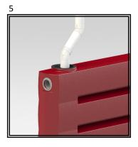
INSTALL DOWNPIPE INTO INLET PREFITTED WITH LEAF STRAINER.
