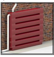
INSTALL OVERFLOW PIPEWORK AND PLUMB AWAY FROM TANK BASE. **NOTE:** FOR MULTIPLE TANKS INLET AND OVERFLOW MUST STILL BE CONNECTED TO THE SAME TANK
