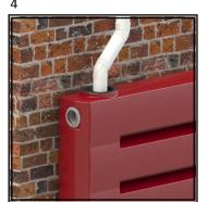
INSTALL DOWNPIPE INTO INLET PREFITTED WITH LEAF STRAINER. EITHER END CAN BE USED
