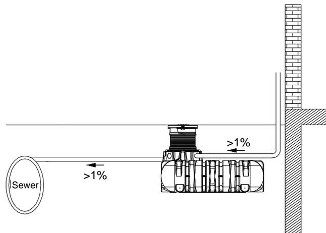
**Important:** The empty pipe must be connected to an aperture **above** the max. water level.
