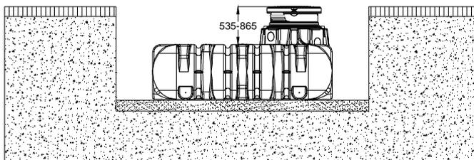
Maximum allowed earth coverage height with second GARANTIA telescopic dome shaft as adapter or extension.
