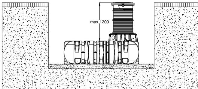
Allowed earth coverage height with GARANTIA telescopic dome shaft and passenger car module with cast iron cover (class B) in areas used by passenger cars (max. total load 3.5 ton).
