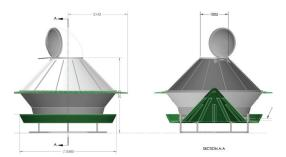
CAPACITY: 9.5m3 DIAMETER: 4,284mm HFIGHT: 2.720mm BASE WIDTH: 3.485mm
